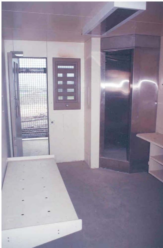
This is a purpose-built, double-occupancy SHU cell with the top bed removed. Door at left rear leads to exercise yard. Door to right accesses shower. Staff control both doors. Desk and toilet areas are at right out of photo.
