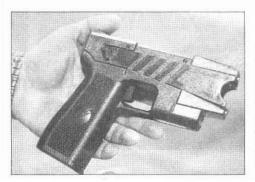
The Taser stun guns are made to look and handle like a regular firearm. Officers can fire up to 21 feet away from the target, and the darts can penetrate up to two inches of clothing.
